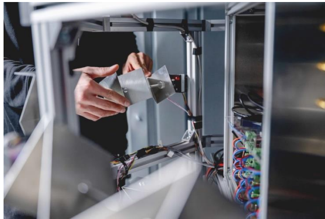
These adjustable mirrors are at the heart of the radio wave technology. Credit: Ruhr-Universität Bochum
