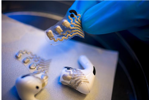
The screen-printed, flexible sensors are attached to the earbuds on a flexible, stamp-like surface. Credit: University of California – San Diego
