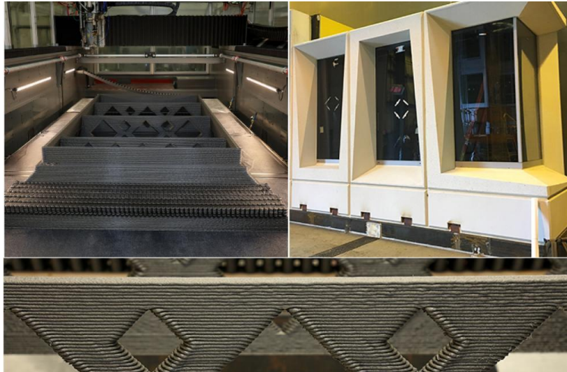
ORNL's 3D-printed polymer composite mold was used to produce precast concrete parts for a New York City building. Researchers conducted a techno-economic analysis that highlights the benefits over wood molds. Credit: Oak Ridge National Laboratory
