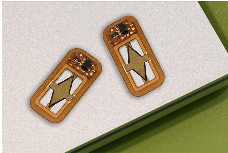
*MIT engineers designed an implantable device that carries hundreds of thousands of islet cells along with its own on-board oxygen factory to keep the cells healthy.*
