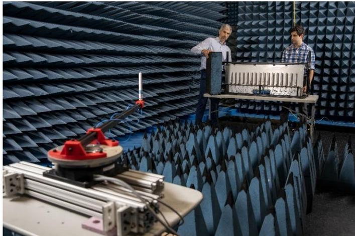
*Final TRIAD demonstration setup, with the transmit antenna in the foreground on a metal arm attached to a turntable and the elemental digital array in the background. Shown are Ryan Westafer and Alex Saad-Falcon.
