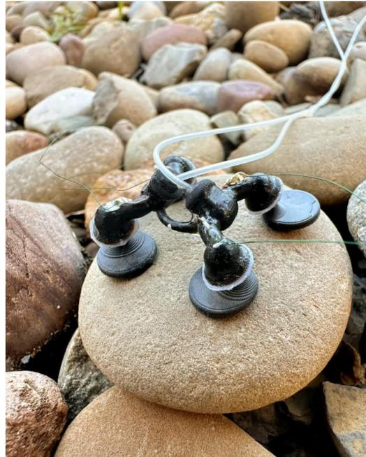
*This combustion-powered quadrupedal robot is capable of multi-gait movements and can leap 60 centimeters in the air, or roughly 20 times its body length.
