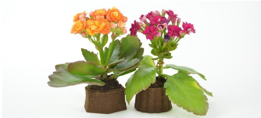
Flower planters 3D printed from used coffee grounds. Credit: Michael Rivera, University of Colorado Boulder
