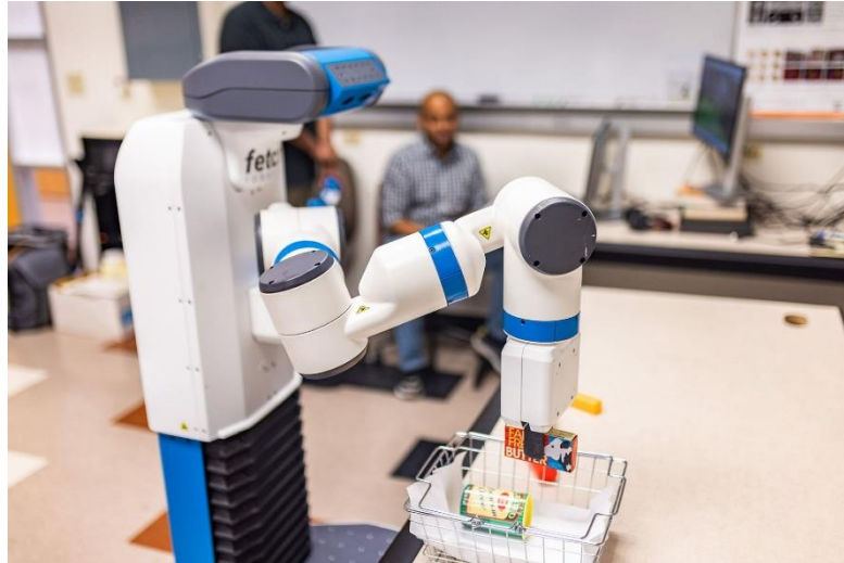
The 4-foot-tall robot has a long mechanical arm with seven joints and a square "hand" with two fingers to grasp objects.
