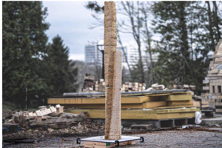
Robotic 3D printing of wood-based material paired with incremental set-on-demand concrete casting to create zero-waste freeform concrete structures.
