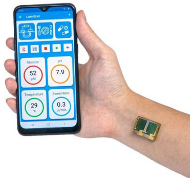
Mobile phone application that pairs with wearable sweat sensor via Bluetooth. Credit: Jihong Min, California Institute of Technology
