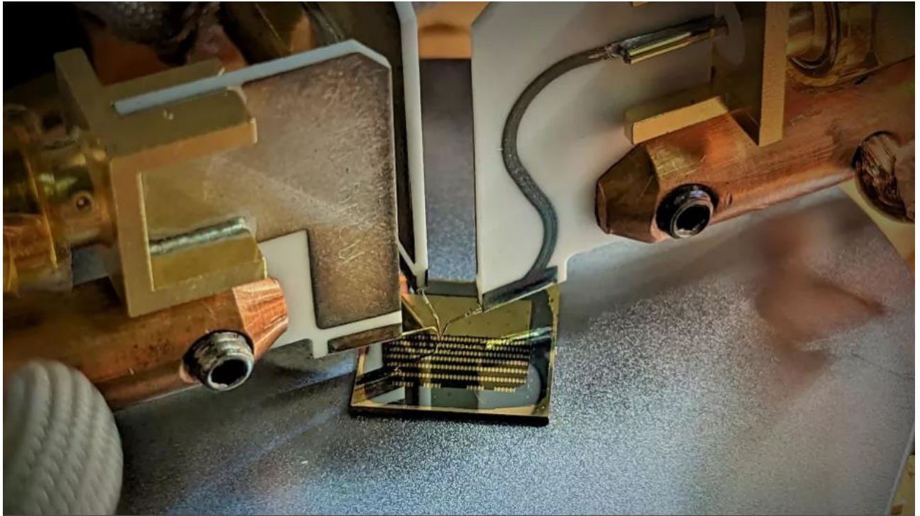
The millimeter-sized chip on which the transistors are located Credit: Anton Persson, Lund University
