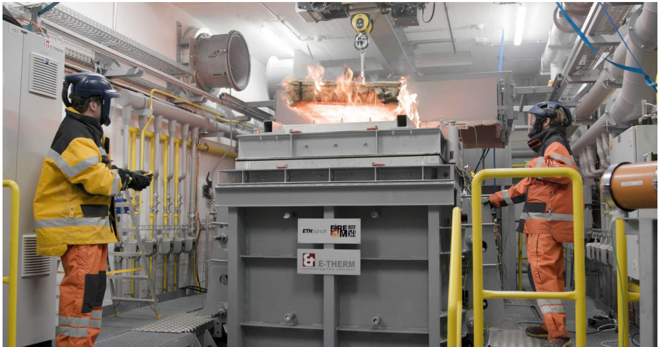
After 90 minutes, the wooden piece is removed from the furnace and extinguished. Credit: Michael Steiner, Eidgenössische Technische Hochschule Zürich
