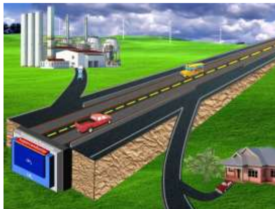
Schematic illustration showing the cross-sectional view of the superconducting highway for energy transport and storage and superconductor levitation for the transport of people and goods in the future.
