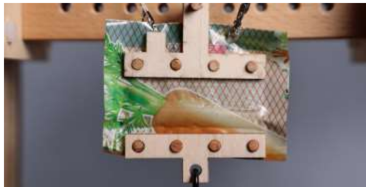
An "artificial muscle" made, in part, from material designed for biodegradable grocery bags. Credit: Max Planck Institute for Intelligent Systems
