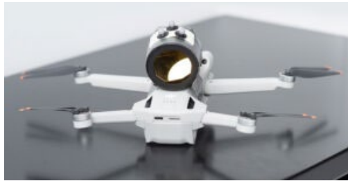
The retroreflector mounted onto the drone. Credit: Bumper DeJesus, Princeton University
