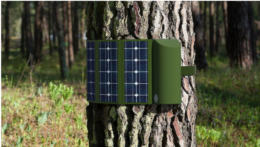
Smart Microphone that can record animal sounds and, with the help of AI, recognize them. Credit: ©Olivier Stähli, École Polytechnique Fédérale de Lausanne
