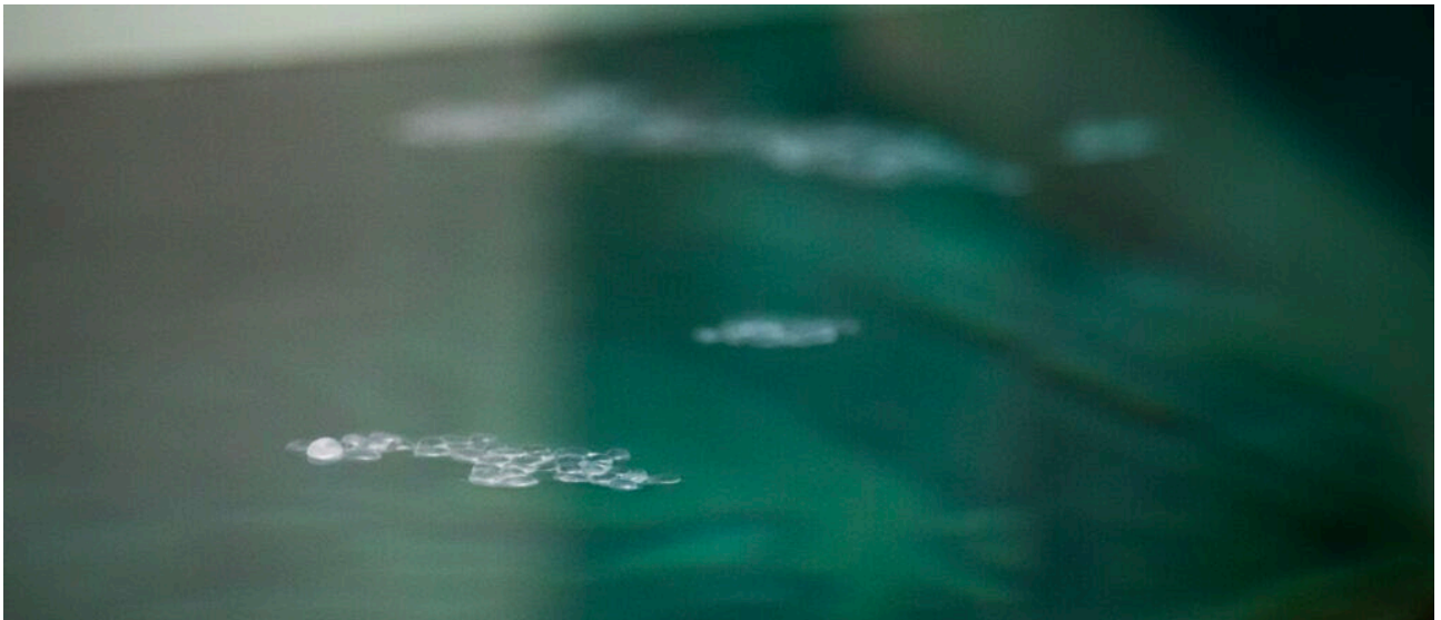
Microplastic pellets float on the surface of water in the wind wave tank at the U-M Marine Hydrodynamics Laboratory as part of a study to determine how they affect measurements of surface roughness.
