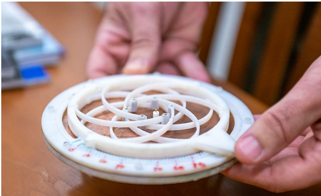
Researchers illustrated and designed a circular, iris-shaped patch antenna prototype using commercial electromagnetic simulation software. Credit: Jeff Xu, Pennsylvania State University
