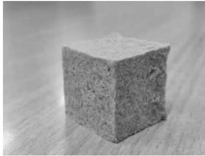
This cardboard-based foam reinforced with gelatin could make packaging materials more sustainable. Credit: American Chemical Society
