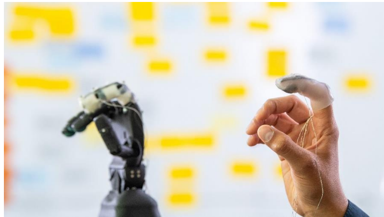
The sensor skin is very flexible and can be attached to many surfaces, including fingers, for example. Credit: Technical University of Munich
