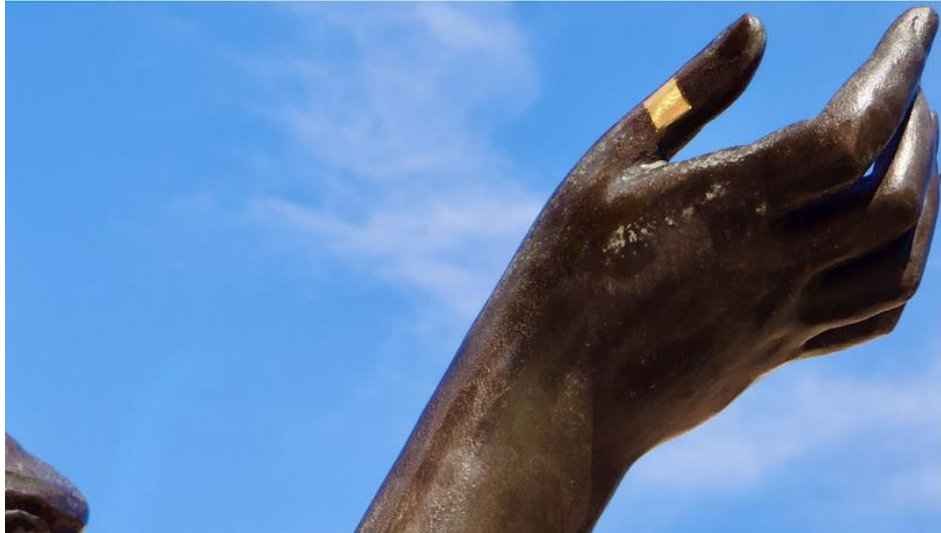
A vIGT array consisting of half a million transistors conforming to the complex curvilinear surface of the finger of Alma Mater, Columbia University's iconic stature. Credit: Dion Khodagholy, Claudia Cea/Columbia Engineering
